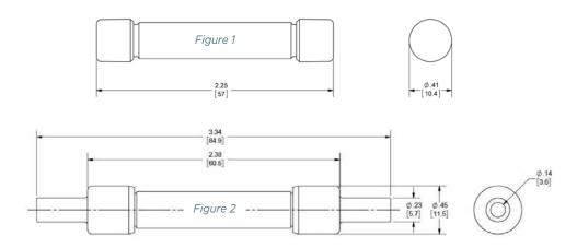
CC terminal (Fig. 2): Recommended crimping tool: T & B Sta-Kon ERG4002 #10 -12 AWG (6-4 mm²)
